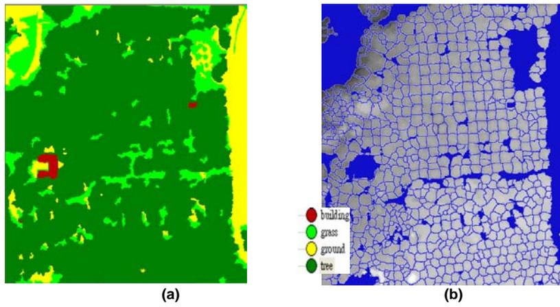
Fig. 6. Segmentation results. (a) classification result of Tai-Chung case, (b) individual tree extraction result of Tai-Chung case
