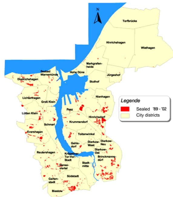
Figure 3: Sealed surfaces in Rostock between 1989 and 2004
