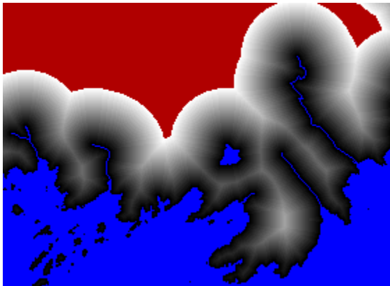
(c) Results following the application of a 40 pixel (1200-meter) buffer from water pixels. Red indicates pixels beyond 40 pixels from water whereas grey variations represent increasing distance from black to white.
