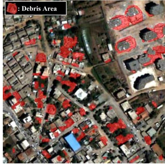
Figure 6. Debris visually detected.
