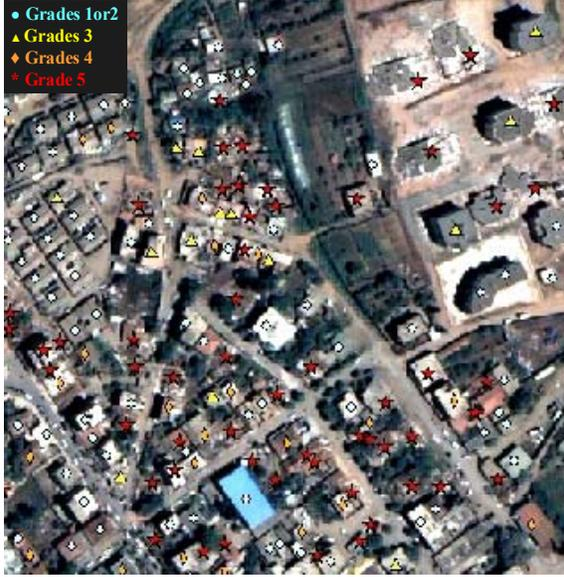
Figure 5. Result of visual building damage detection.
