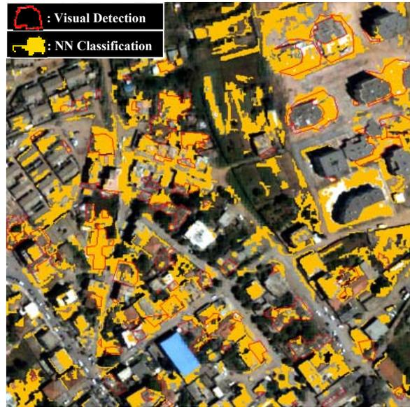
Figure 8. Debris detection by the object-based approach
