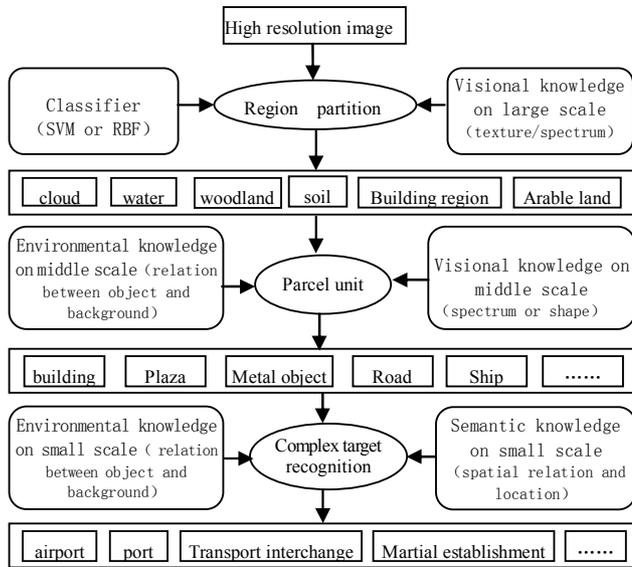
Figure 1. Work flow of multi-scale information extraction from high resolution remote sensing images based on features
