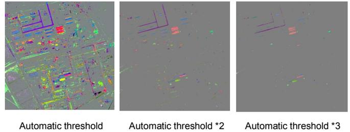
Figure 3. MAD components 1 (red), 2 (green) and 3 (blue) with (increased) automatically estimated threshold
