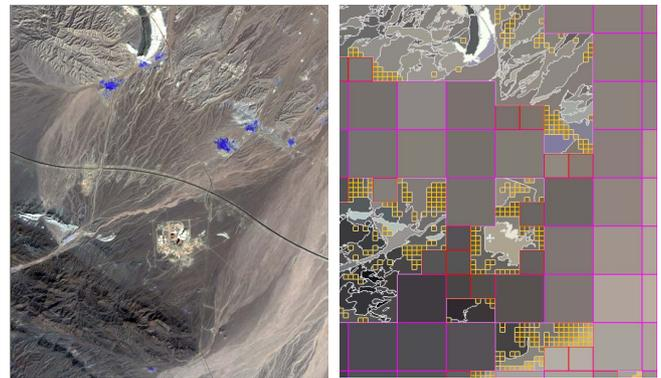
Figure 1. Extract of AST07, green (R), red (G), NIR (B) over Natanz (left) and its chessboard/multiresolution segmentation, level 6 (right)
