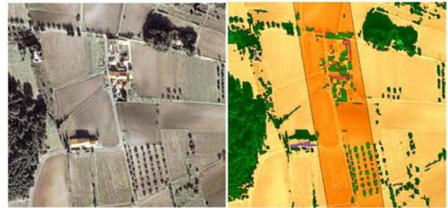
Figure 2 Identification of objects near a pipeline track based on 1 m resolution IKONOS images. The right image contains the eCognition object classes separated into areas inside and outside the surveillance corridor
