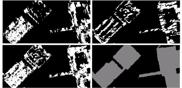
Figure 3. Classification comparison. (top left) East-West pass, (top right) North-South pass, (bottom left) Combined building class, (bottom right) Reference data
