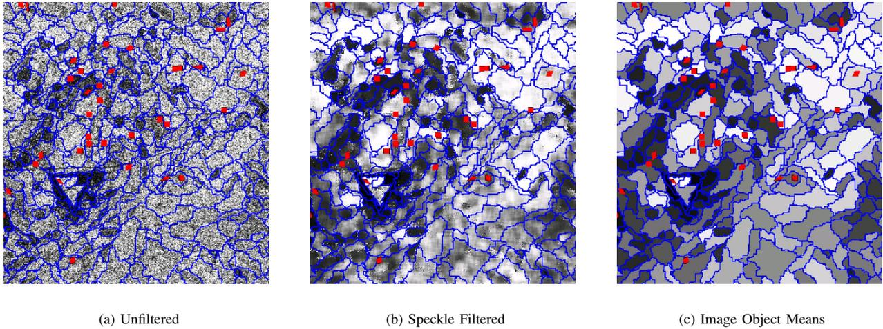
Fig. 1. Segments generated from joint ERS/JERS segmentation shown overlaid on JERS data in the Raco test site.
