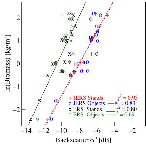
Fig. 3. Comparison of biomass regression models derived from stand and image object backscatter values.
