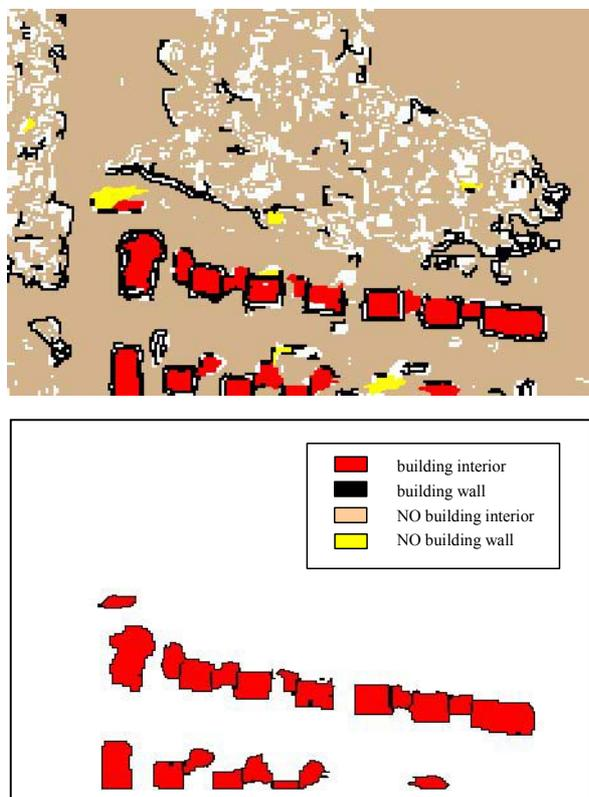
Figure 3. Classification of building elements (top) and result after post-processing (bottom).
