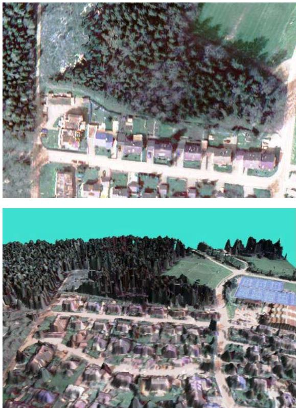
Figure 1. Part of the multi-sensoral data set: Multi-spectral imagery (top, coverage approx. 400 m x 300 m) and perspective view after draping onto the Digital Surface Model (bottom).
