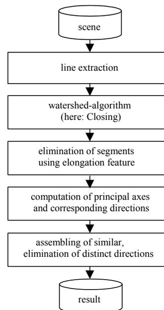
Figure 4. Simple algorithm (bottom) for the extraction of area structures (top right) from given imagery (top left: near IR channel, coverage approx. 160 m x 420 m).
