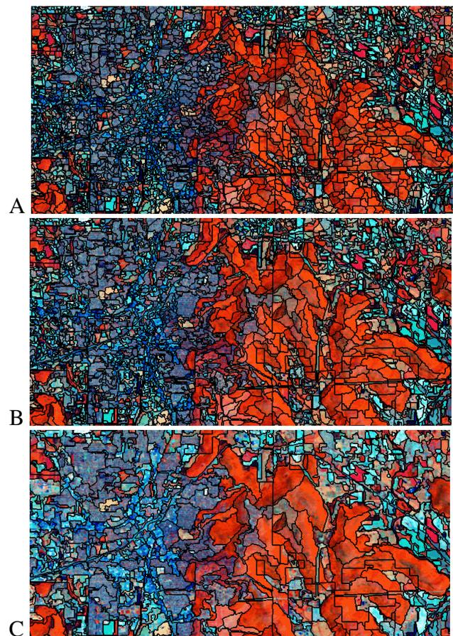
Figure 2. Image segmentation using three different scale parameters Scale parameter A= 5, B=15, and C=25
