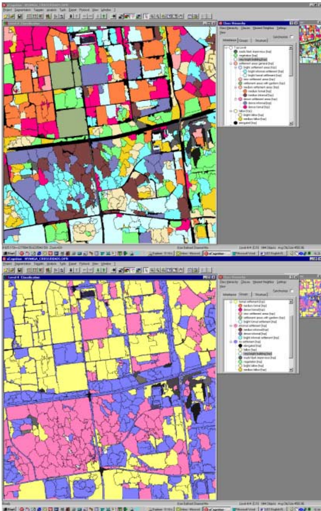
Fig. 10: Grouped (bottom) and ungrouped (top) classification result of level 4. Note: Some non-settlement segments remained unclassified.
