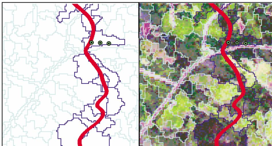
**Figure 2.** Illustration of segments with lidar data (dark blue), segments with no lidar data (light blue), a SLICER flight line (red), and some field plots (green/black circles). The two panels show the same segment information, but the right panel has the Landsat-5 TM (red, green, infrared) data as a backdrop to illustrate the segmentation results.
